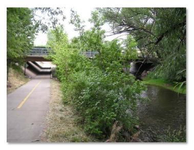
**Photograph 10-9**. Striping used sparingly can be effective in alerting the user of a safety concern. In this photo, it is used where the path approaches a crossing.
