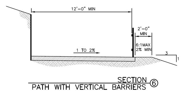
Figure 10-6. Path section with vertical barriers on both sides
