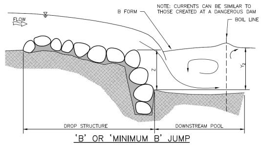
THIS FORM CAN BE BENIGN OR CREATE A PLUNGING OR DIVING JET (AS ILLUSTRATED) THAT CAN BE OVERLY-RETENTIVE AND HAZARDOUS. THIS IS OFTEN CAUSED BY A LOWER THAN PREDICTED TAIL WATER ELEVATION ( $\gamma_2$ ) OR DOWNSTREAM DEGRADATION OF THE CHANNEL OR RIVER BED.
