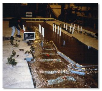
**Photograph 10-35.** A physical model aided in the 1996 design of Confluence Park. This was one of the first whitewater venues to employ the hydraulic jump at an abrupt drop design. As a result, the venue performed well over a very wide range of flows for a diverse user group. Photo courtesy of McLaughlin Whitewater Design Group.
