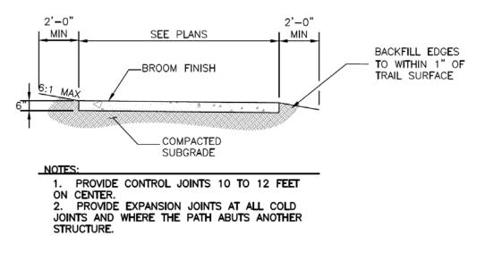
Figure 10-10. Concrete path section
