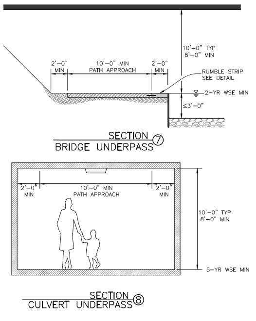
Figure 10-7. Path underpass sections
