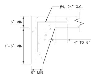
Figure 10-1. Thickened edge detail
