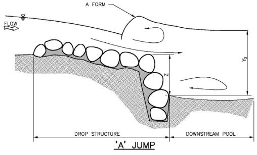
THE A JUMP IS CREATED IF THE TAILWATER IS HIGH AND IS USUALLY UNAVOIADABLE THROUGHOUT THE ENTIRE RANGE OF RIVER FLOWS. THIS CONDITION CAN BE SOMEWHAT RETENTIVE AND POWERFUL, BUT NOT NECESSARILY HAZARDOUS.
