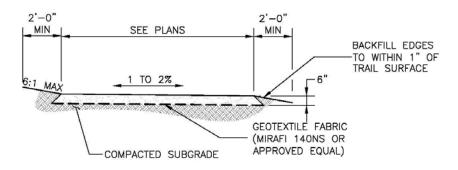
Figure 10-9. Crusher fines path section
