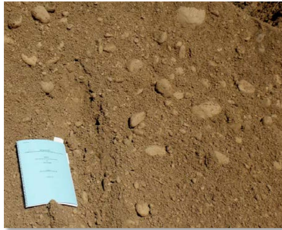
Photograph 8-20. Four-inch minus pit run surge is also an important ingredient to fill gaps between riprap.
