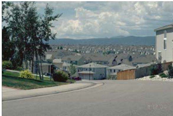
Photograph 6-2. Urbanization (impervious area) increases runoff volumes, peak discharges, frequency of runoff, and receiving stream degradation.
