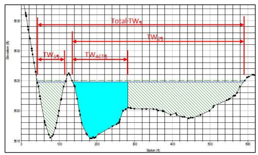
Total Top Width (TW) includes high ground and ineffective flow areas.  $TW_1$  could be an adjacent on-site detention pond.  $TW_2$  includes the Actual Top Width ( $TW_{ACT}$ ) and an ineffective flow area caused by a downstream embankment.
