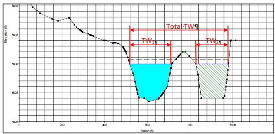
Total Top Width (TW) includes high ground and ineffective flow area (TW<sub>2</sub>) Actual Top Width =  $TW_1$
