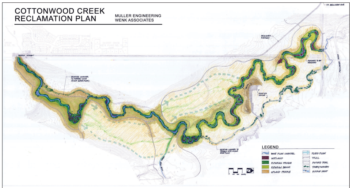
Figure 4. The Cottonwood Creek Project created a meandering base flow channel with rock riffles and pools and adjacent wide overbank areas where high flows can spread out to dissipate energy. The project, emulating a natural floodplain stream, was constructed by the Cherry Creek Basin Water Quality Authority to help protect Cherry Creek Reservoir.
