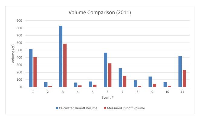
Figure 2 - Calculated vs. Measured Volume Storm Event Comparisons (2011)
