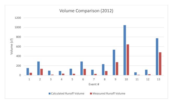
Figure 3 - Calculated vs. Measured Volume Storm Event Comparisons (2012)
