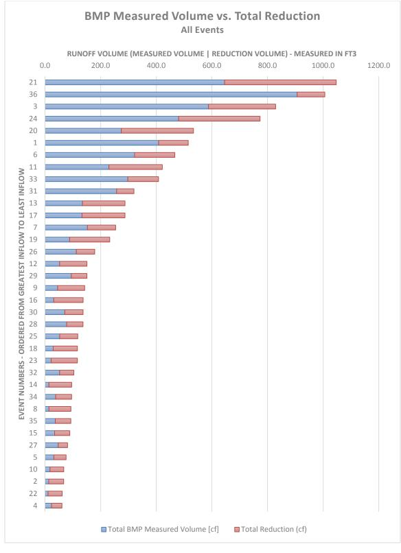
Figure 7 - Summary of BMP Measured Volume vs. Reduction Volume (ordered by greatest to least inflow)
