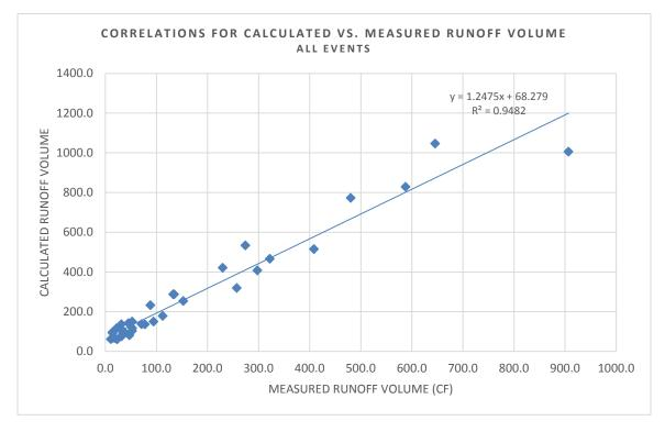
Figure 6 - Correlation for Calculated vs. Measured Runoff Volumes (all years)
