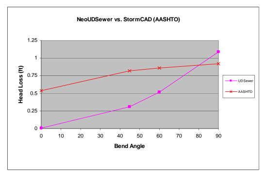
Figure 1 – Head loss results as a function of bend angle for UD-Sewer and StormCAD
