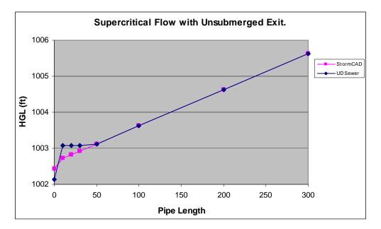
Figure 3 - Supercritical Flow with Unsubmerged Exit
