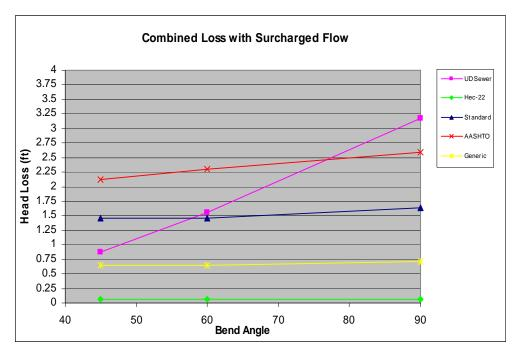
Figure 11 – Combined Loss with Surcharged Flow
