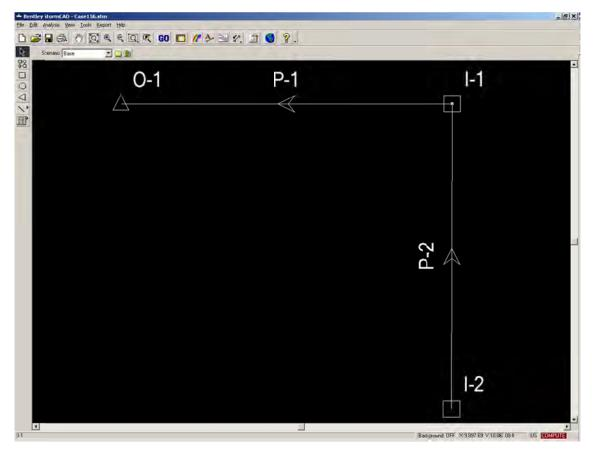
Figure 12 - Screenshot from StormCAD, this storm sewer system has 2 pipes that link at the I-1 Junction and bend 90 degrees. At the Junction point, double click to enter edit mode.
