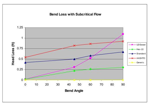
Figure 7 - Bend Loss with Subcritical Flow
