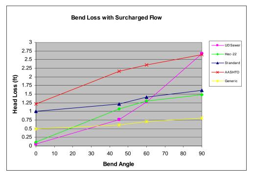
Figure 8 - Bend Loss with Surcharged Flow
