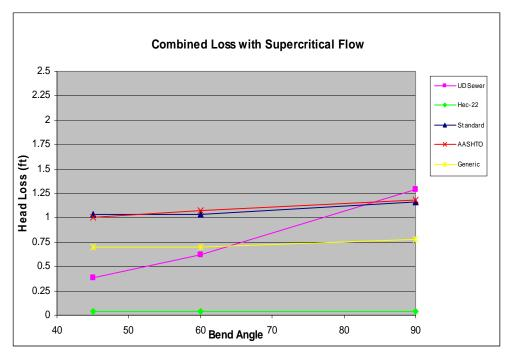
Figure 9 - Combined Loss with Supercritical Flow
