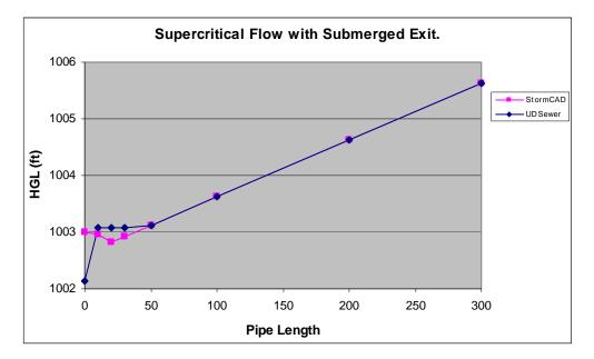
Figure 5 - Supercritical Flow with Submerged Exit
