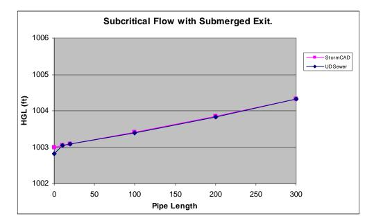
Figure 4 - Subcritical Flow with Submerged Exit
