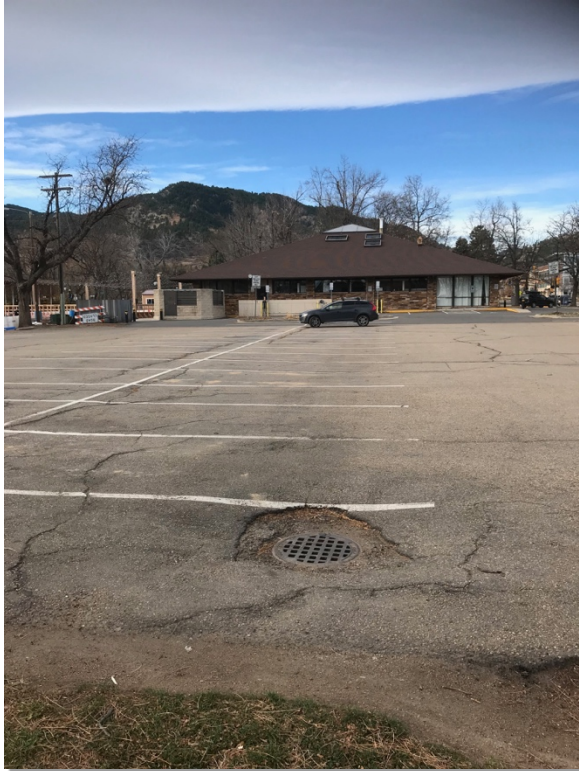
Photograph 3-1. Separate Pervious Area (SPA) is permeable but does not receive runoff from impervious areas, such as the tree lawn in this photo. The drive and street are examples of DCIA.
