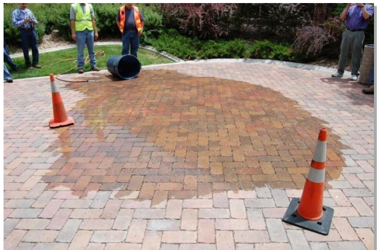
Photograph PICP-8. The limits of wetting remain the same after multiple demonstrations.
