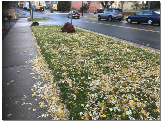
Photograph 3-1. Separate Pervious Area (SPA) is permeable but does not receive runoff from impervious areas, such as the tree lawn in this photo. The drive and street are examples of DCIA.
