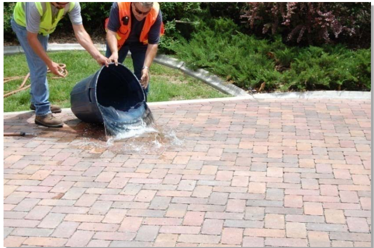
Photograph PICP-7. City staff demonstrate the infiltration capacity of PICP at the Greenwood Village City Hall.
