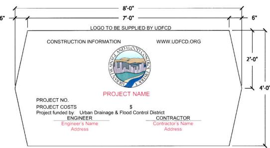
SIGN TO BE ON 3/4" MARINE PLYWOOD AND HAVE A PALE GREEN BACKGROUND WITH BLACK LETTERING. EMBOLDED LETTERS ARE 3" HIGH, ALL OTHERS ARE 2" HIGH. POSTS SHALL BE 4" X 4" CEDAR WOOD. SIGN SHALL BE ATTACHED TO POSTS WITH (4)-1/2" X 3" LAG BOLTS.
