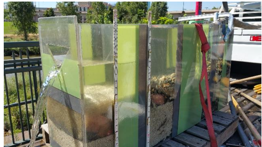
Treatment Systems Being Pilot Tested in Denver
