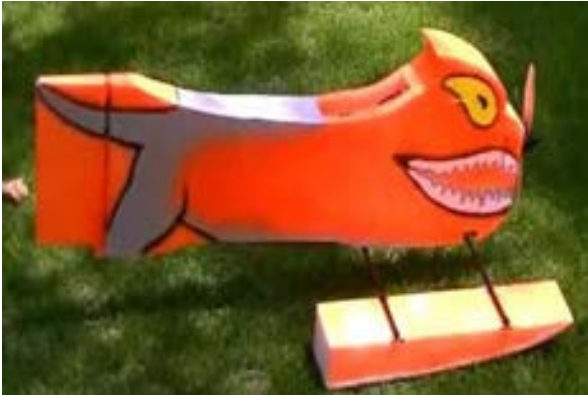
Remote controlled goose hazing device, "Goosinator," used to deter resident waterfowl in Denver Parks.
