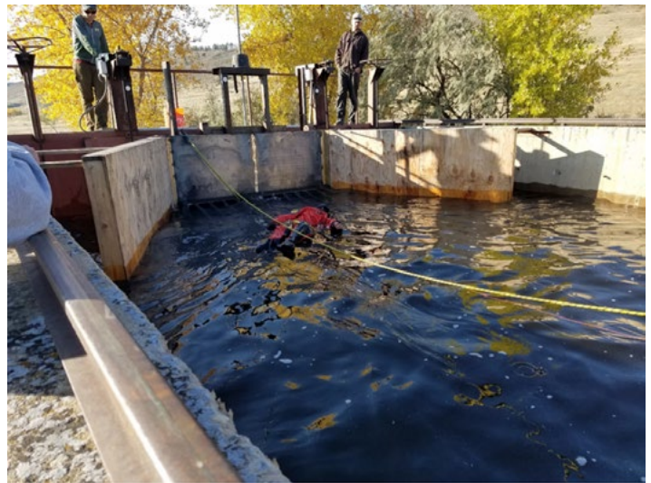
Members of the Larimer County Dive Rescue Team use a safety mannequin for initial testing at the CSU safety grate physical model.
