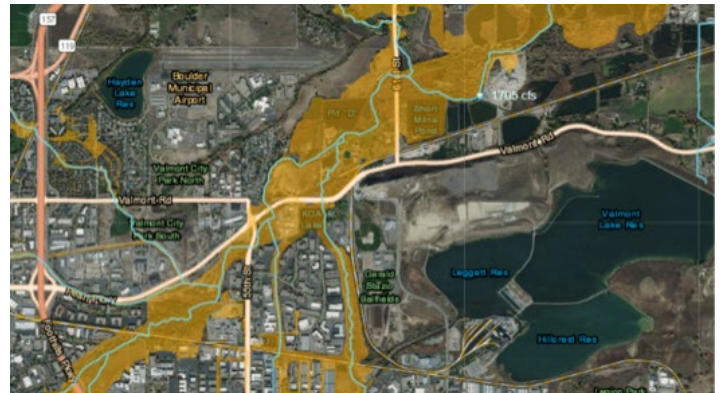
Peak flow estimates and approximate flood extents from the 2013 Flood Peak Estimates map.
