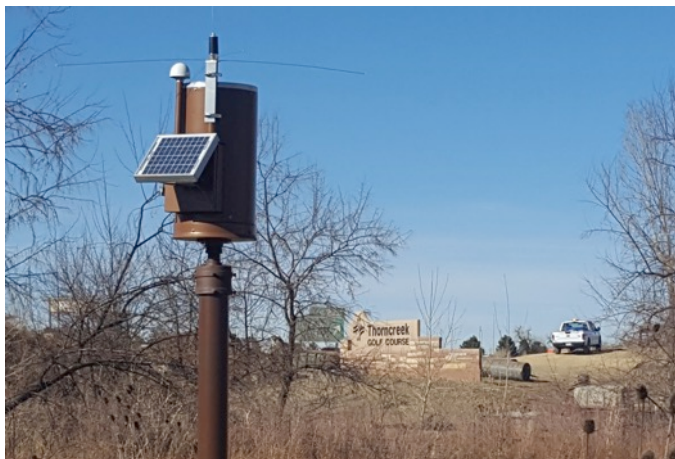
New rain/stream gage on Big Dry Creek at Thorncreek Golf Course in Thornton
