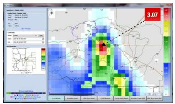
Gage Adjusted Radar Rainfall (GARR) estimates for the August 30, 2016 storm located over Boulder Creek about 2 miles west of Boulder
