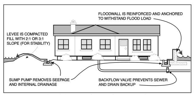
Figure 4-10. Example of levee and floodwall protection
