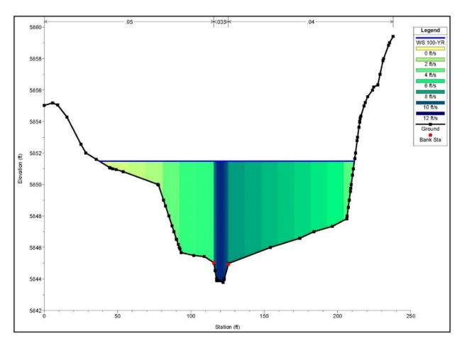
Figure 8-31. Example HEC-RAS cross section with velocity distribution
