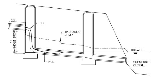
Figure 7-12. Hydraulic and energy grade lines
