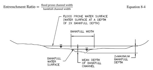
Figure 8-12. Channel cross section with bankfull and flood prone water surfaces (Rosgen 1996)
