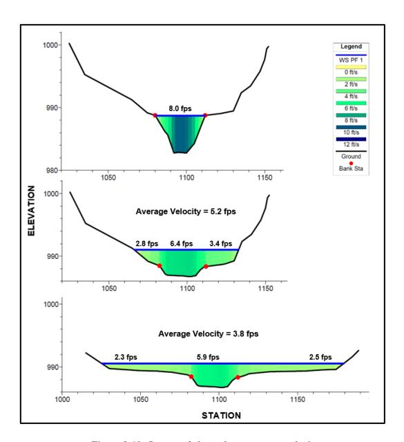
Figure 8-10. Impact of channel geometry on velocity
