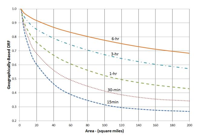
Figure 5-2. Depth reduction factor (DRF) curves for minor storm events (2-, 5-, and 10-year events)
