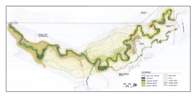
Figure 8-15. Example of meandering single-thread channel form (Courtesy: Wenk and Associates)
