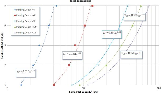
Denver No. 16 Combination Inlet Interception Capacity based on depth of ponding (depth measured outside local depression)
