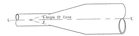
Figure 7-15. Angle of cone for pipe diameter changes
