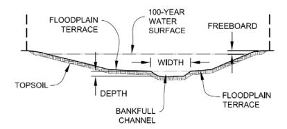
Figure 8-21. Typical naturalized channel geometry
