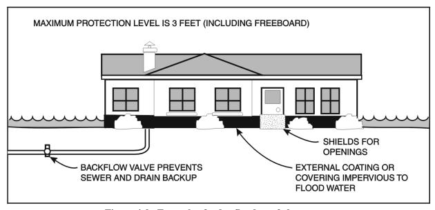
Figure 4-9. Example of a dry floodproofed structure
