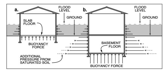
Figure 4-4. Buoyant force and hydrostatic pressure diagram
