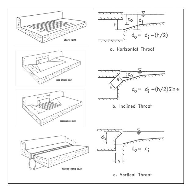
Figure 7-9. Perspective views of grate and curb-opening inlets
