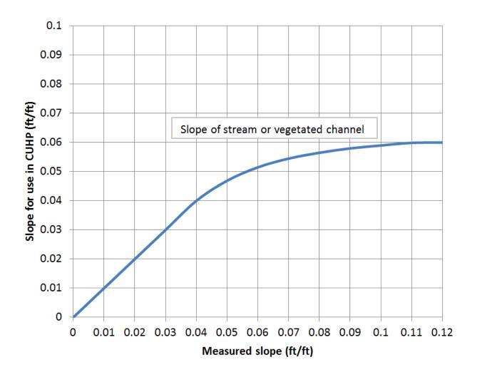
Figure 6-4. Slope correction for streams and vegetated channels
