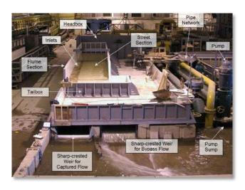
**Photograph 7-1.** From 2006 to 2011, hundreds of street and area inlet physical model tests were conducted at the CSU Hydraulics Laboratory, facilitating refinement of the HEC-22 methodology for inlets common to Colorado.
