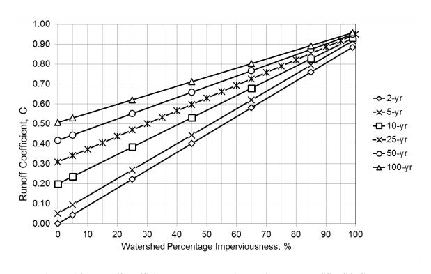
Figure 6-3. Runoff coefficient vs. watershed imperviousness NRCS HSG C and D
