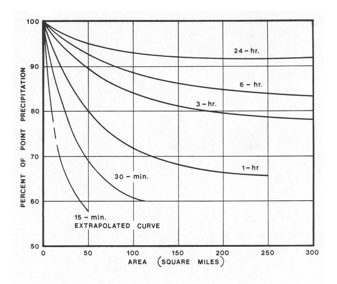
Figure 5-1. Depth reduction factor (DRF) curves for infrequent storm events
