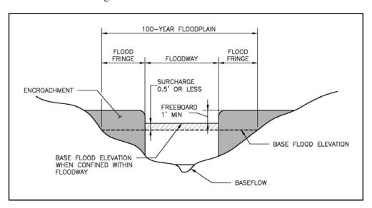
Figure 4-1. Floodway and flood fringe
