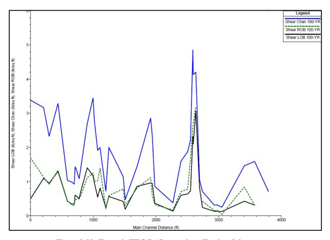
Figure 8-32. Example HEC-RAS general profile plot of shear stress
