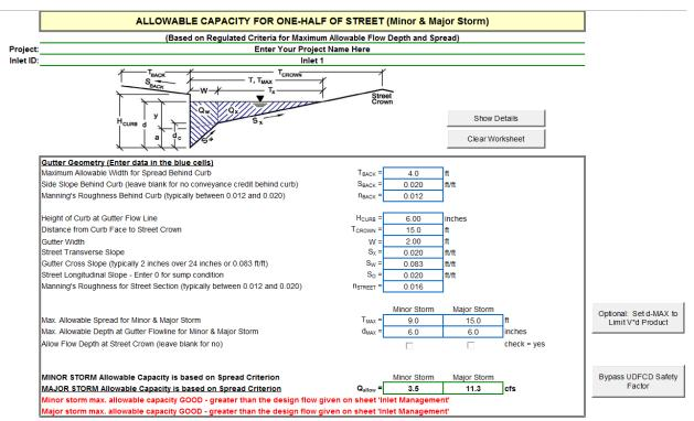
The screenshot below shows the inlet design specifications. Notice that there is bypass flow for both storms. These flows will be accounted for at the next (downstream) inlet. The length of the inlet or number of units can be increased to reduce bypass flow.
