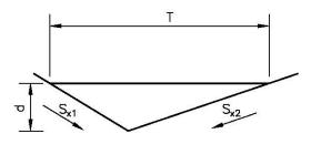
Figure 7-5. Typical v-shaped swale section
