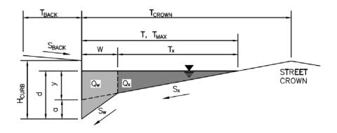
Figure 7-2. Typical gutter section—composite cross slope
