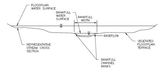
Figure 8-11. Channel cross section with bankfull discharge illustration
