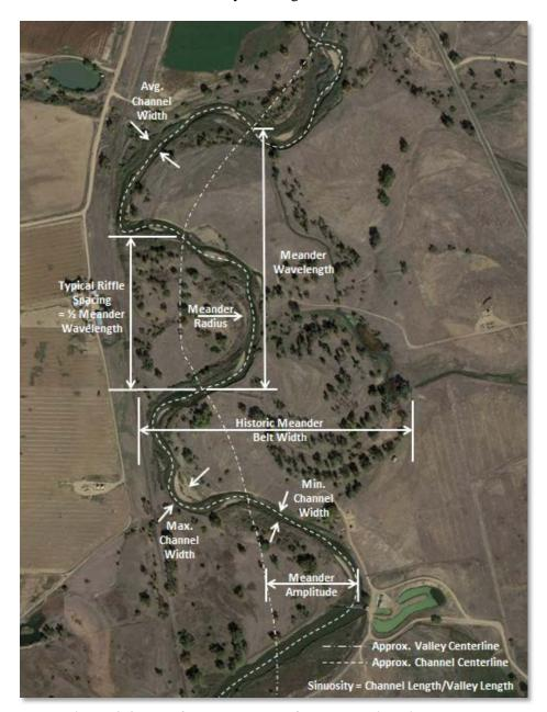
Figure 8-8. Planform geometry of a meandering river system
