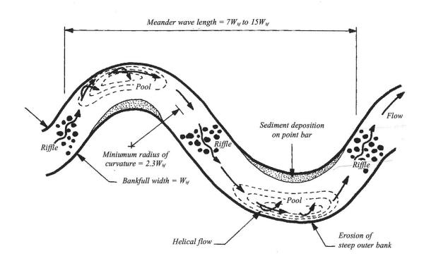
Figure 8-14. Riffle-pool stream form
