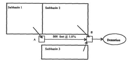
**From Subcatchment 1:** The flow time includes the time of concentration of Subcatchment 1, and the flow time from Point A to Point B through the street. The flow time from Subcatchment 1 to Point B is the sum of the time of concentration of Subcatchment 1 and the flow time through the 500-foot gutter:
