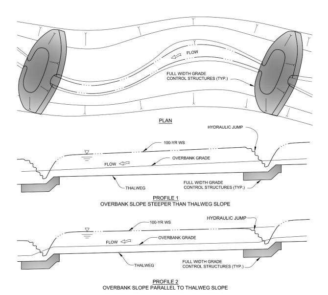
Figure 8-16. Full width grade control structures
