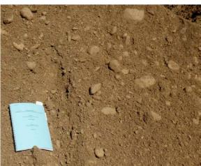
**Photograph 8-19.** Seven-inch minus crushed surge is a key ingredient to fill gaps between riprap.
