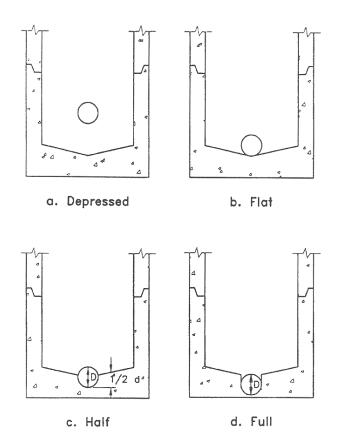
Figure 7-14. Manhole benching methods
