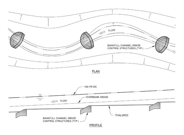
Figure 8-17. Bankfull channel grade control structures
