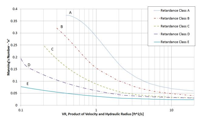
Figure 8-28. Manning's roughness in vegetated channels
