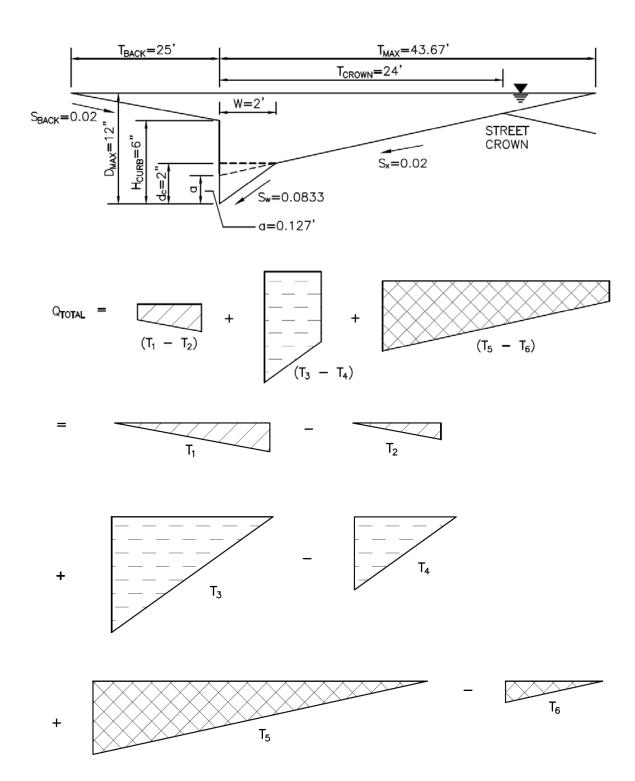
After flow in each of the 6 triangles has been determined, add and subtract the flow in each area as shown in the above figure.
