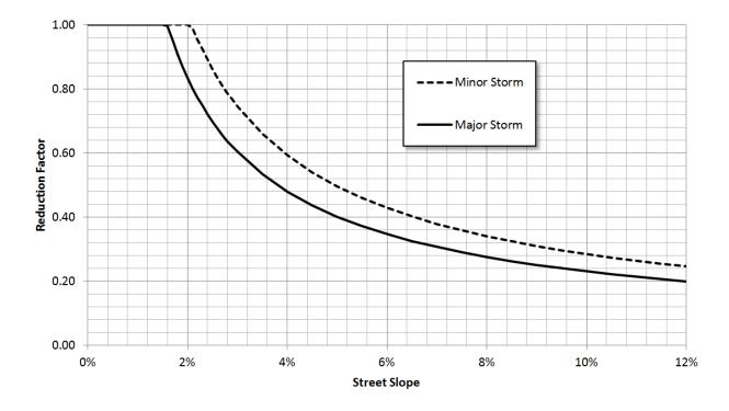
Figure 7-4. Reduction factor for gutter flow (Guo 2000b)
