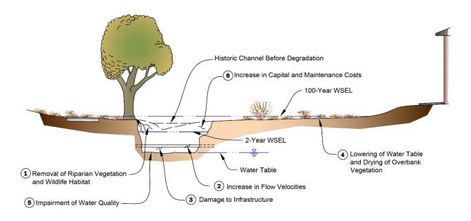
**Figure 8-5. Impacts of stream degradation** (Source: Arapahoe County)
