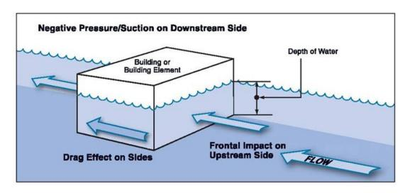
Figure 4-6. Effects of moving water on a structure
