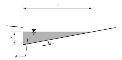
Figure 7-1. Gutter section with uniform cross slope
