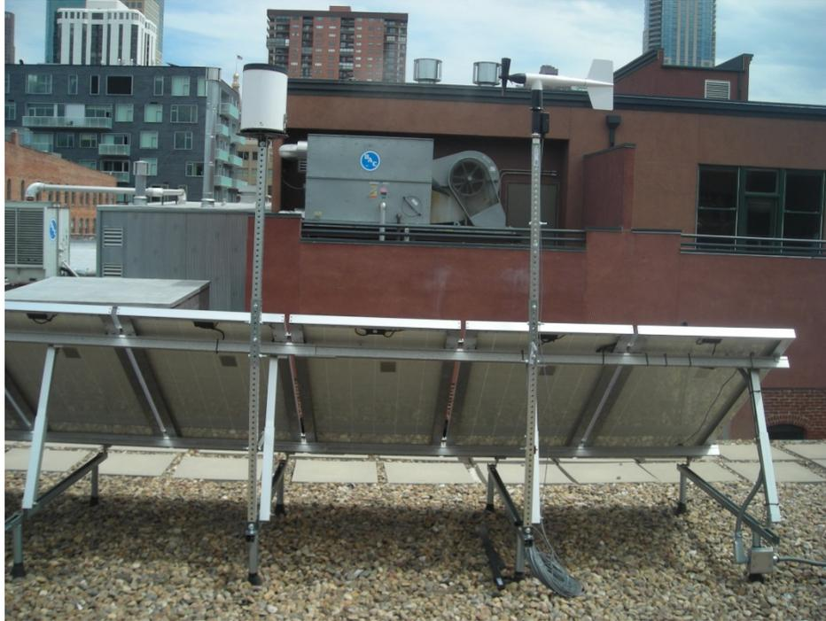
**Figure 1 - Rain Gage and Anemometer located on rooftop of Alliance Center**
