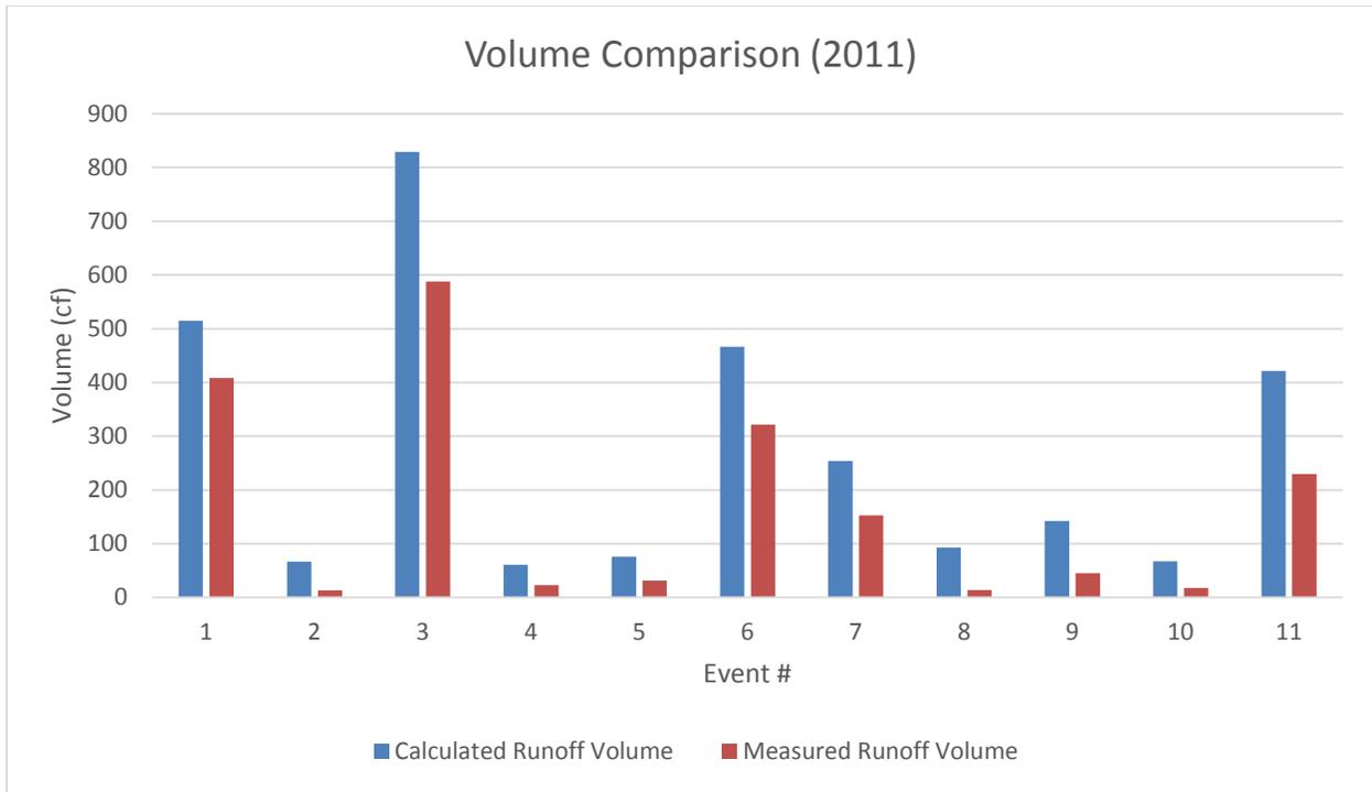
**Figure 2 - Calculated vs. Measured Volume Storm Event Comparisons (2011)**
