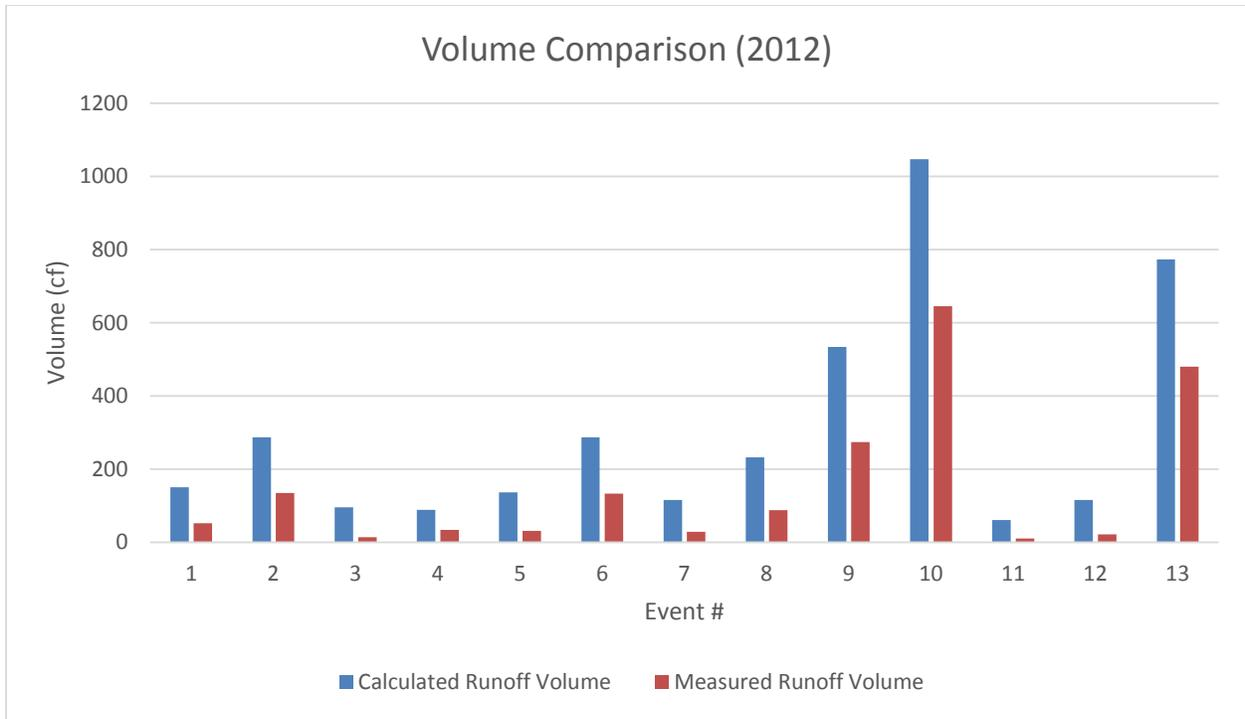
**Figure 3 - Calculated vs. Measured Volume Storm Event Comparisons (2012)**
