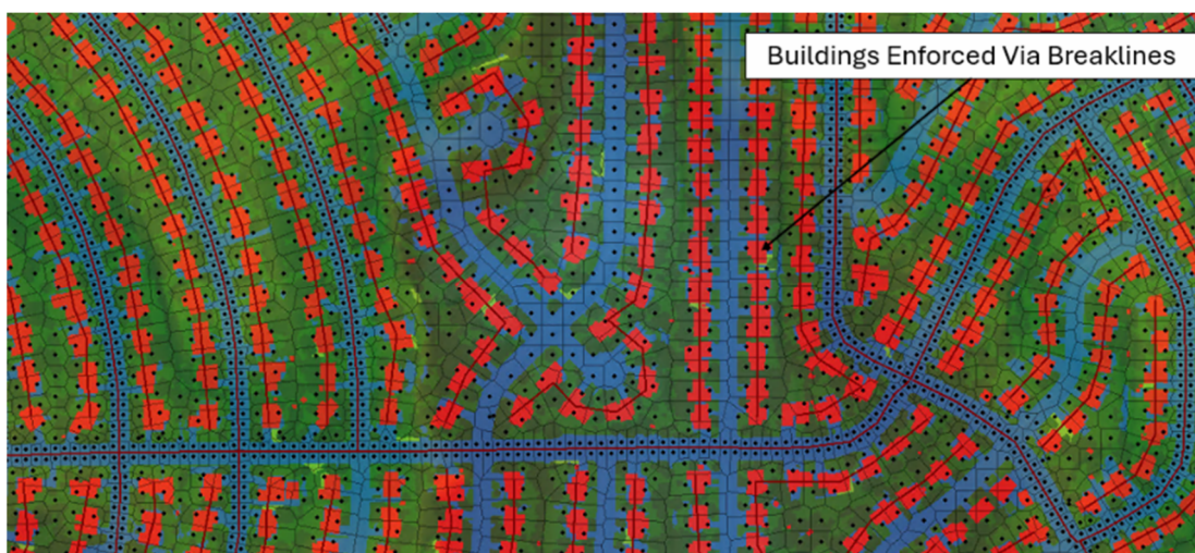
Figure 23. Example of Buildings Enforced with Breaklines in an Urban Area
