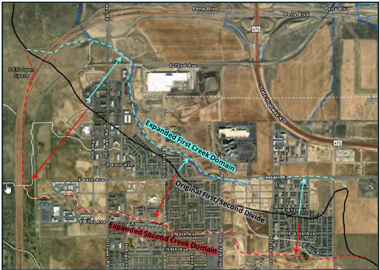
Figure 7. Example Need for Domain Expansion and Overlap due to Uncertain Flow Paths
